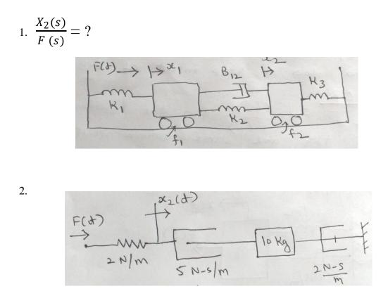
Write equation of motion of translational system as shown above and determine Transfer function.
